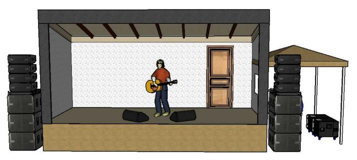
Stage Deck: Stage Height: Roof Trim Height: 20' wide X 8' deep 30" inches 10' ft from deck
